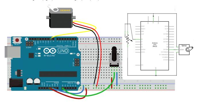
Note: Servos can draw significant current. If you need to control more than one or two servos, use an external power supply instead of the Arduino's +5V pin.
